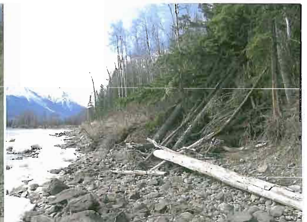
Photo 37: View downstream at typical distorted vegetation, irregular ground and eroded banks along toe of landslide.
