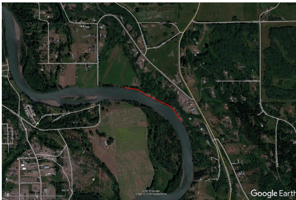
Figure 32: Recommended Erosion Protection Extent
