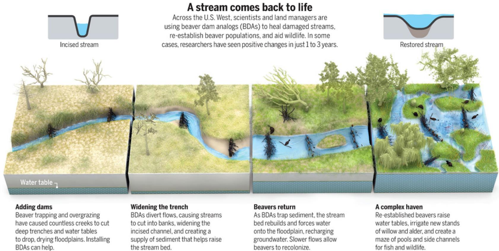
Figure 7. Illustration of using Artificial Beaver Dams to help rejuvenate a stream.
