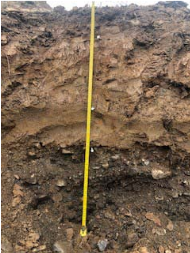
Soil pit as described in 2021 showing 65cm silt cap over 60+% gravels with sand matrix.
